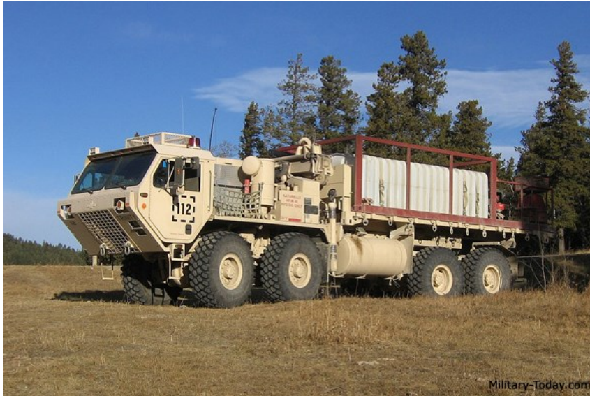
M1120 Oshkosh HEMETT LHS: Solution to add troop transportation kit to the flatrack
