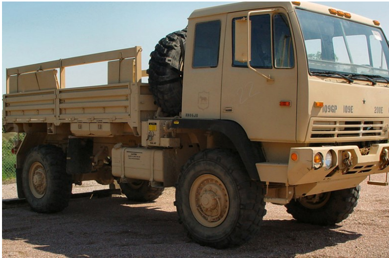
M1078 with troops seats similar to kit that would be added to a flatrack
