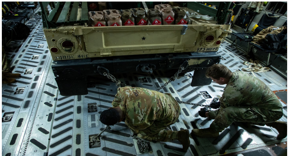
Soldiers from the 573rd Engineer Company securing the chain tie-downs of the vehicle onboard a USAF C-17. (Photo by XVIII Airborne Corps PAO)
