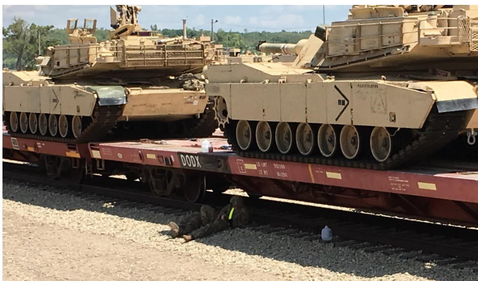
Soldiers violating railhead safety rules by laying under railcars. SDDCTEA Modal Instruction 19 Rail, Section X, Safety Checklist states “Remind soldiers to stay alert no sleeping, resting, or standing around, under, on, or between railcars”. (Photo by: Ken Lewandowski)
