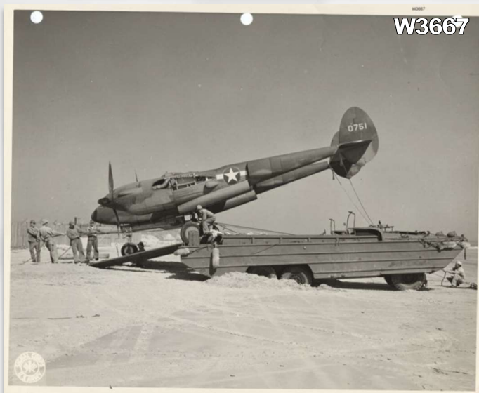
IMAGES W3665, W3666, W3667 - A series of Army Signal Corps photos showing the cross-loading of an assembled P-38 aircraft during transport from a larger ship to two DUKW for transfer during JLOTS operations during training at Fort Story, Virginia in 1943. Source: Army Transportation Museum W03665-W03667
