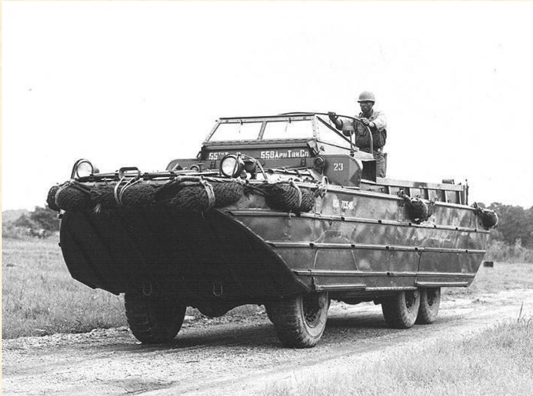
***The DUKW was an amphibious version of the 2-1/2 ton General Motors cargo truck. It was developed by the U. S. Army during World War II as a means to deliver cargo from ships at sea, directly to shore.***
