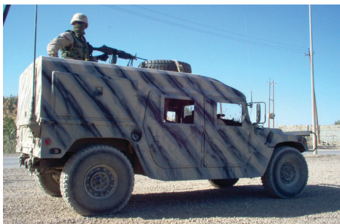
Zebra gun truck before the .50 caliber machine gun was added. At the time of the ambush it had no door armor.
