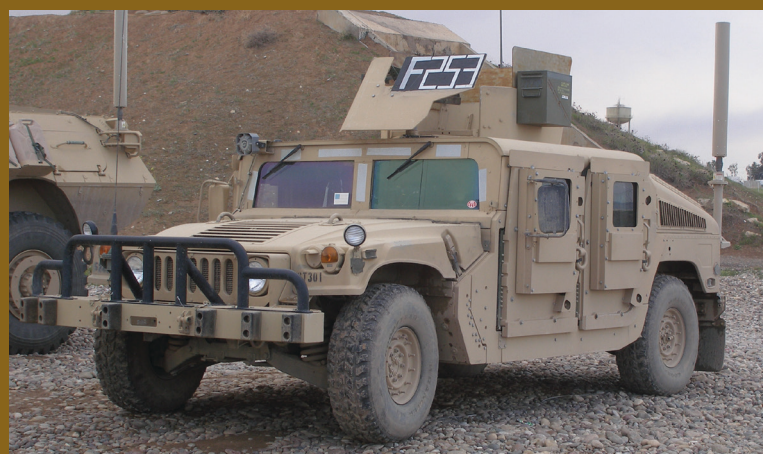
Top: M1151A1 with Rhino 2, Dukes jammer, AM General Gunner Protection Kit, Marine Corps gun shield, and extra ballistic glass on turret and door.
