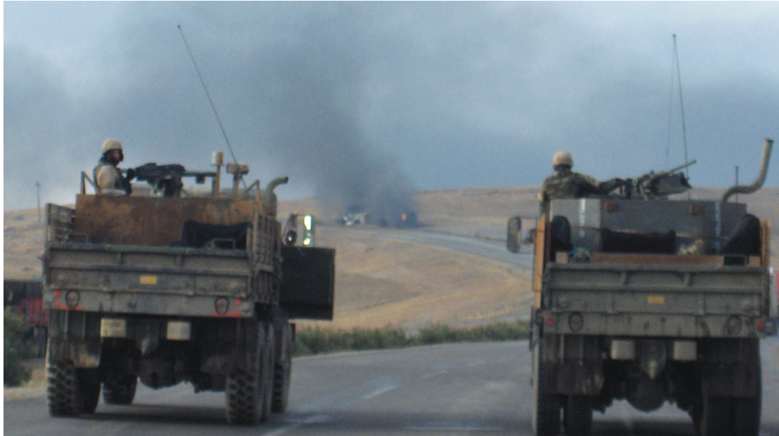
M923 5-ton gun trucks with gun boxes designed by Skunk Werks.
