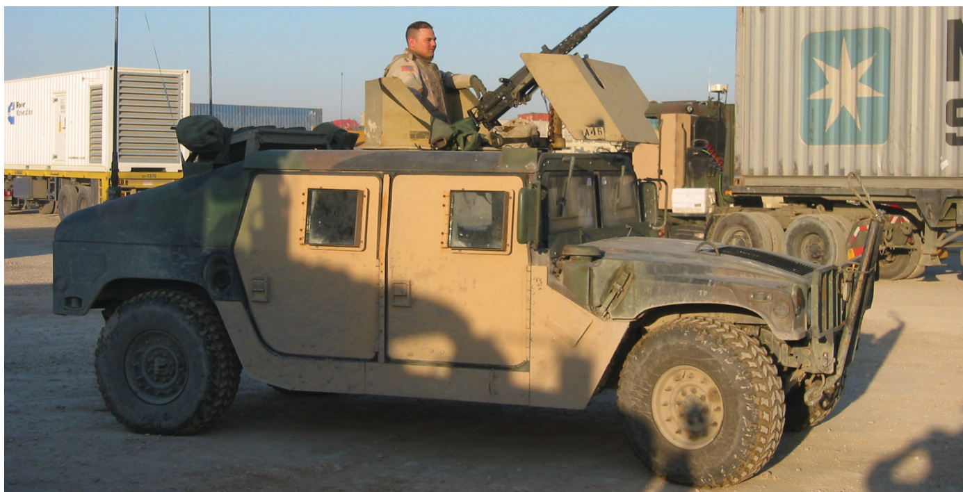
HMMWV of the 1-178th FA with add-on armor kit, local purchased turret armor and gun shield. They escorted the 1LT Kleiman's HET convoy. Photo courtesy of the Richard Killblane
