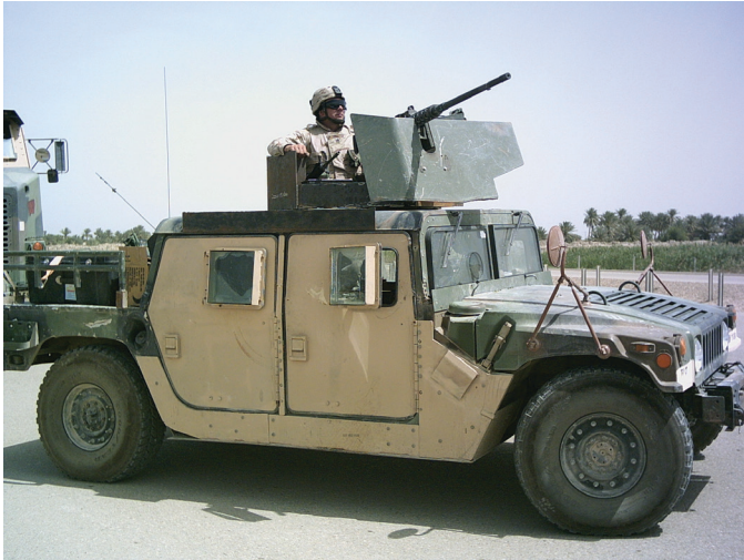
Add-on-Armor Kit on M998 HMMWV of the 1158th Transportation Company (HET). Photo courtesy of 1158th Transportation Company
