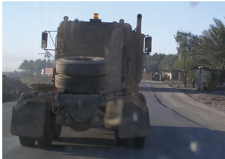
M915 bobtail truck at the end of the convoy. These spare tractors were used to pick up a trailer from a disabled M915.
