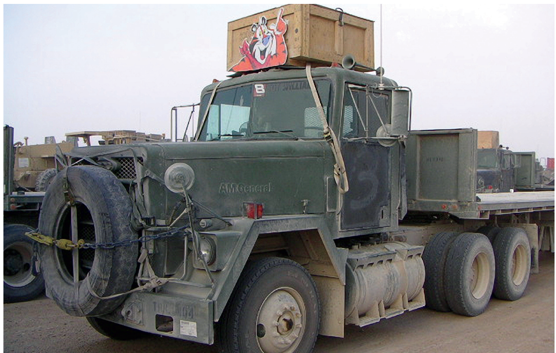
M915 tractor with steel plate welded to the door. Photos courtesy of 518th GT Company
