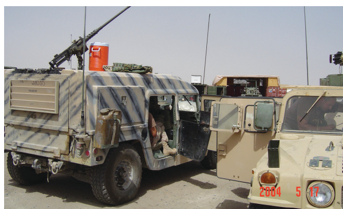
Top: Pedestal mount for the .50 caliber machine gun was added to the Zebra right before the mission.
