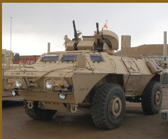
Top: M1151A1 with Rhino 2, Dukes jammer, AM General Gunner Protection Kit, Marine Corps gun shield, and extra ballistic glass on turret and door.
