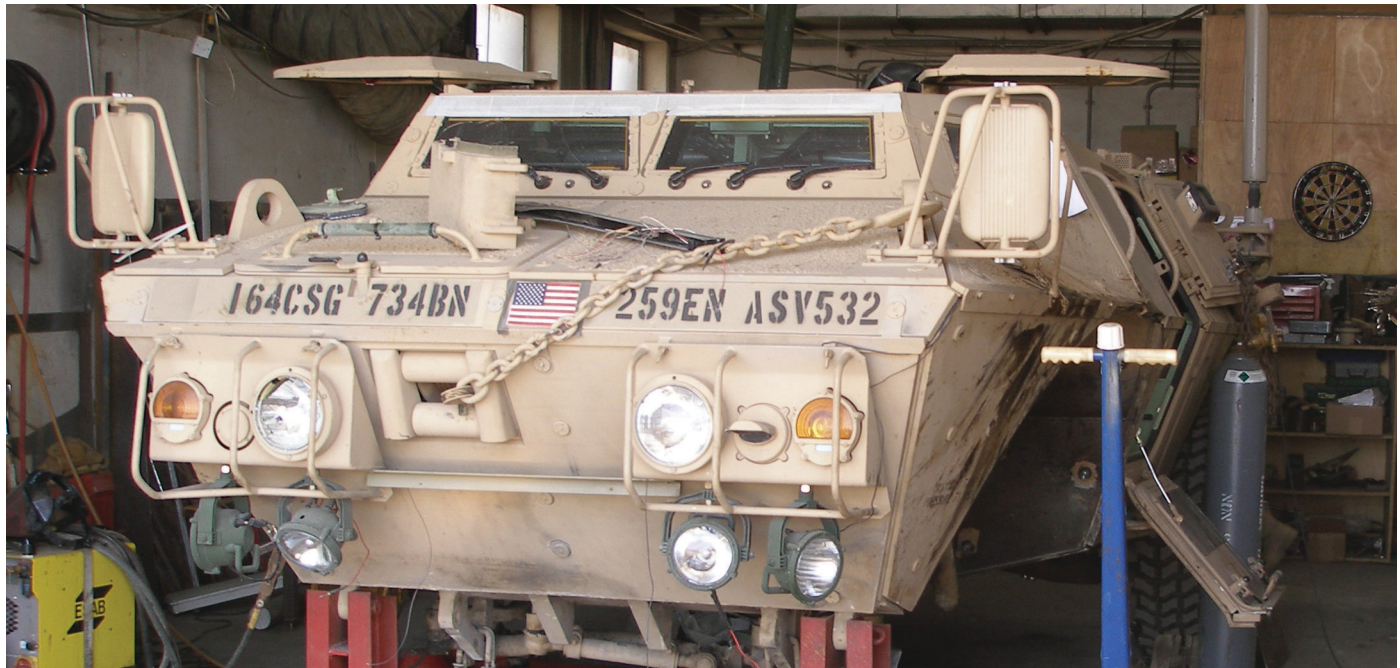
Skunk Werks patching and adding additional armor to underside of M1117 ASV. Photo courtesy of Richard Killblane
