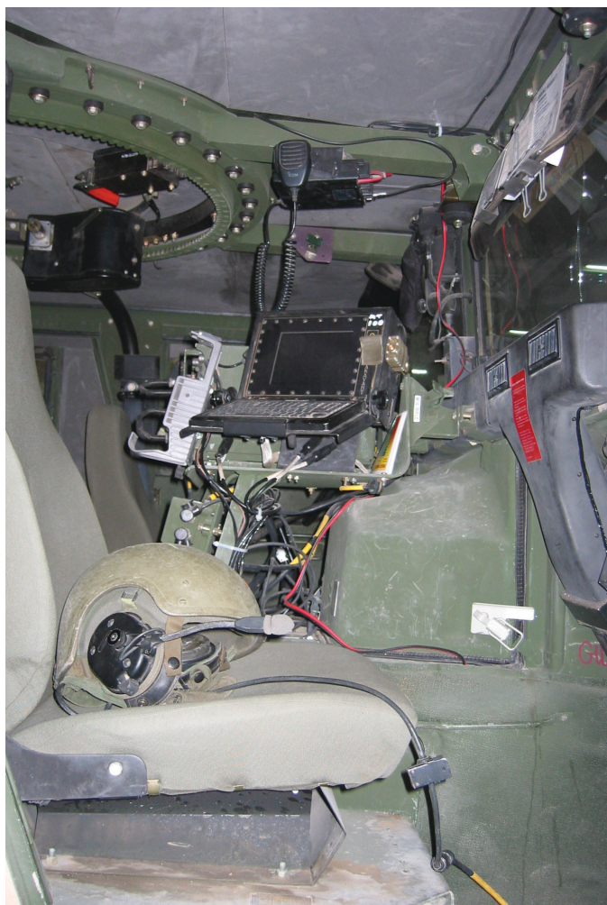
MTS laptop display and CVC helmet with internal communications. Photo courtesy of Richard Killblane
