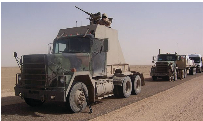
Later view of the M915 gun truck, but with a .50 caliber machine gun instead of the Mk19. Photo courtesy of the 518th Gun Truck Company
