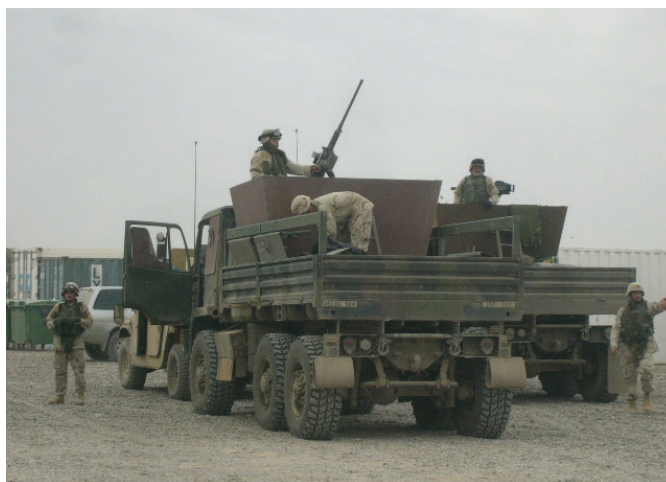
M1083 FMTV 5-ton gun trucks of the 25th Transportation Company with Tea Cup design gun box. Photo courtesy of Pablo Santiago
