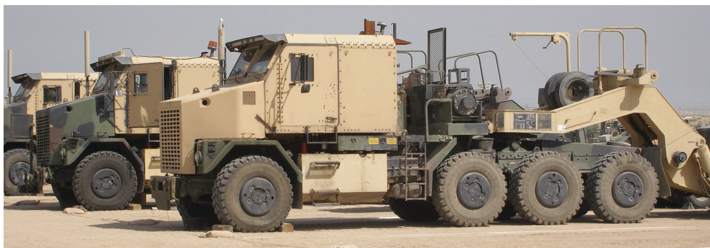
The new cab armor kit for the M1070 HET tractor. The white antenna is the Dukes electronic jamming device used to jam radio signals for arming or detonating IEDs. Photo courtesy of Richard Killblane
