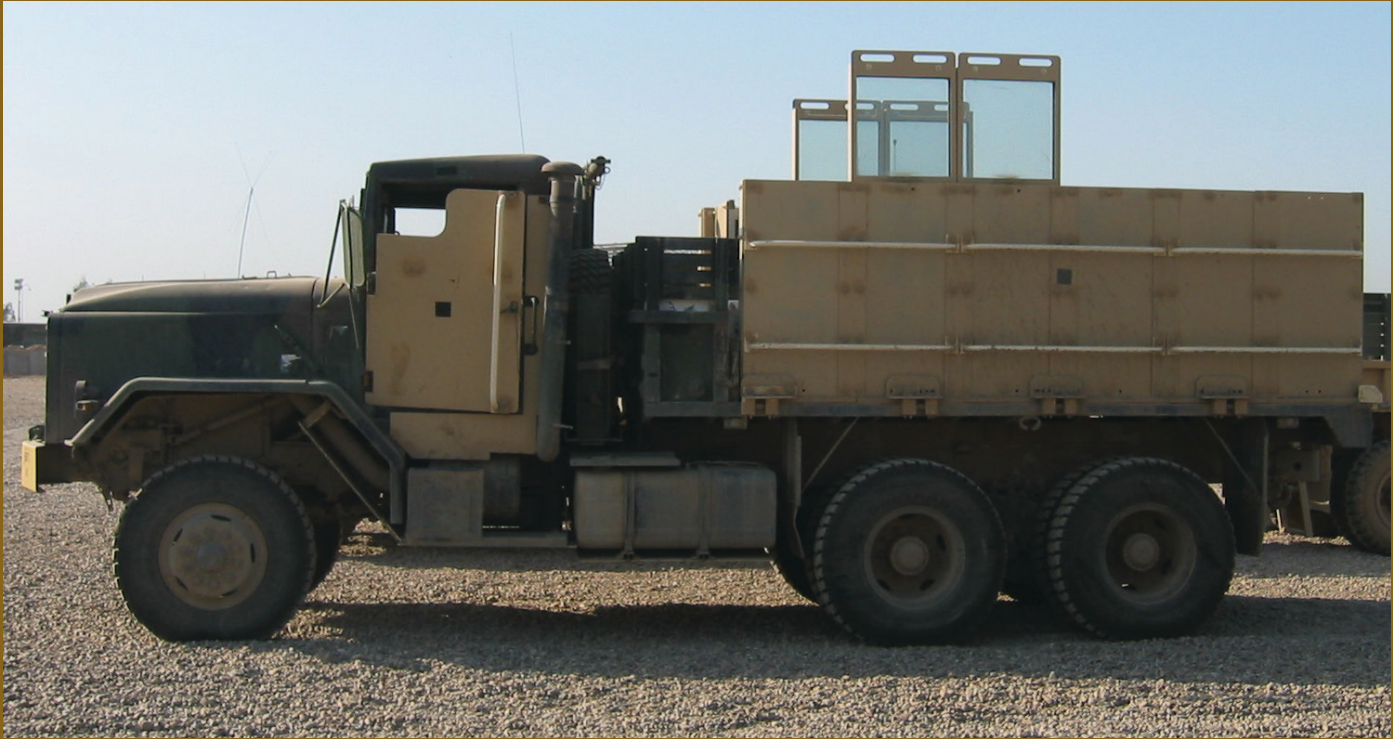
M923 with Lawrence Livermore National Laboratory (LLNL) gun box prior to the policy excluding gunners in the back. Photo courtesy of Richard Killblane
