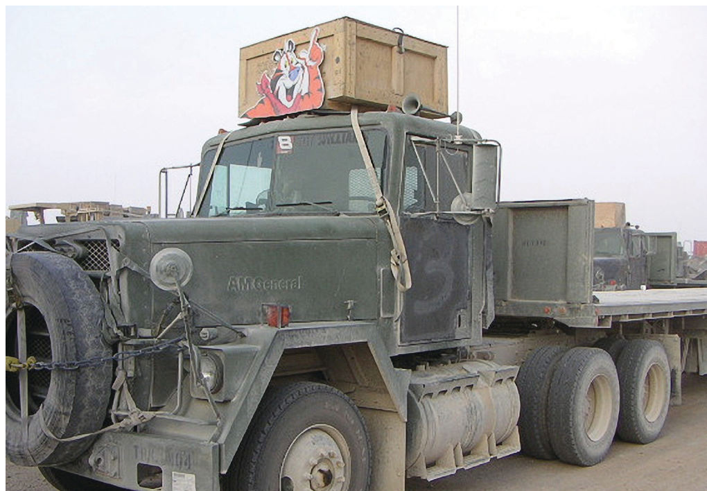
M915 tractor with sheet metal door armor. Photo courtesy of the 518th Gun Truck Company
