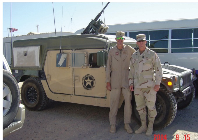
CPT Robert Landry and SGT Jon Henley standing next to a M998 HMMWV gun truck with turtle shell top and mount for M2 .50 caliber machinegun. The 518th painted a marshal's star logo on their doors. Photo courtesy of Robert Landry
