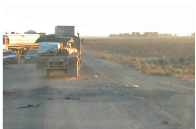
IED crater on ASR Cheyenne shook loads loose on trailers. Photos courtesy of the 1173rd Transportation Company
