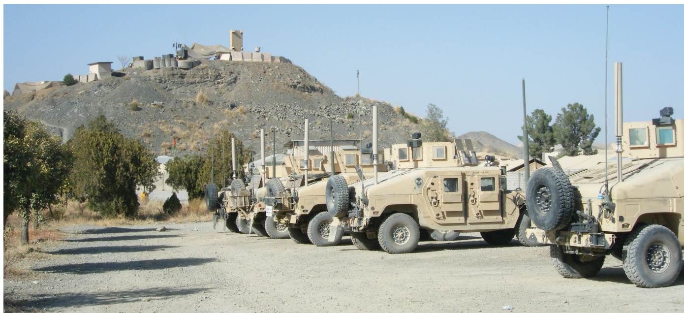
M1114s with Frag 5 doors and Dukes belonging to the 782nd BSB at FOB Salerno. Photo courtesy of Richard Killblane
