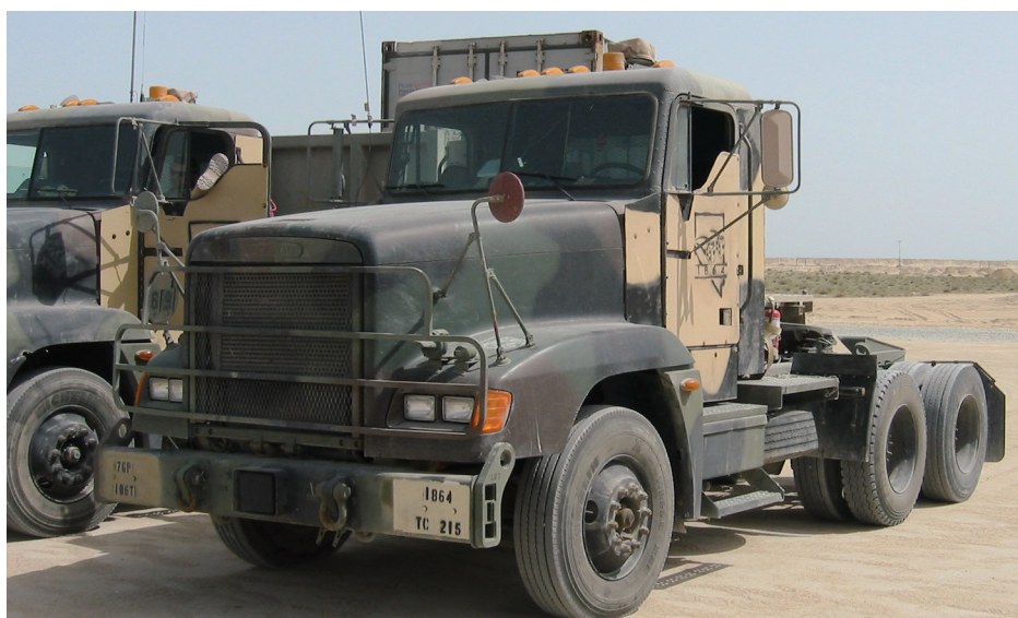
M915A3 of the 1864 Transportation Company. It had the same improvised door armor as the 1075th. Photo courtesy of Richard Killblane
