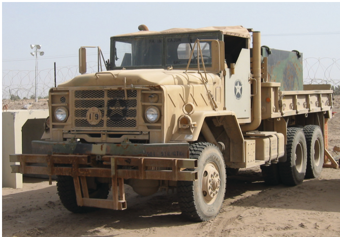
“Big O” was a M923 5-ton gun truck with a pushing bumper designed for busting through road blocks.
