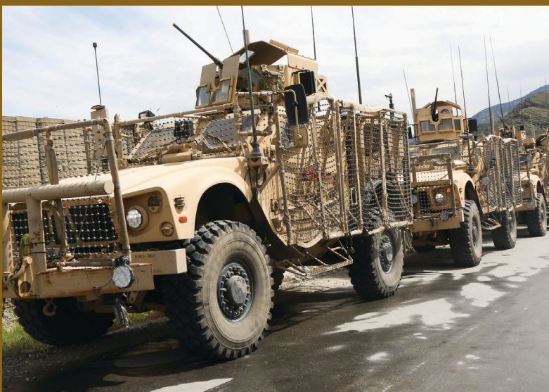
Bottom Left: MRAP All Terrain Vehicle (M-ATV) with anti-RPG Q-net. Photo courtesy of SPC Vang Seng Thao DVIDS
