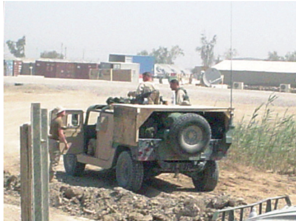
SSG Thomas Stewart's M998 HMMWV gun truck with add-on armor kit. Photo courtesy of Thomas Stewart
