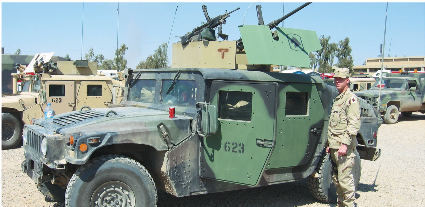
M1114 of the 623rd Field Artillery had dual weapon systems, M2 .50 caliber machinegun and M249 SAW.
