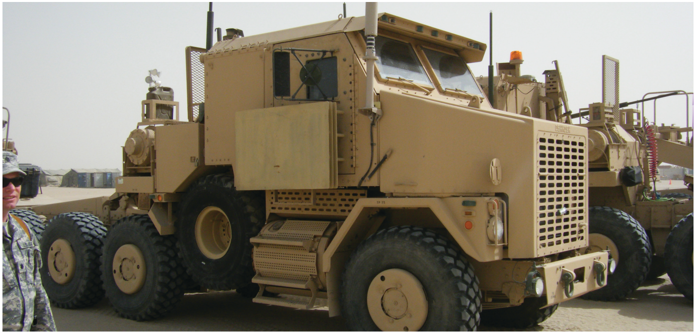
Realizing the HET was the most survivable vehicle against an IED or EFP, convoys started leading with a HET tractor with additional door armor to protect against an EFP. Photo courtesy of Richard Killblane
