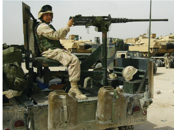
OIF 1 Sit and Spin design HMMWV gun truck of the 1836th Transportation Company (HET). Photo courtesy of Stephen Ruggiero
