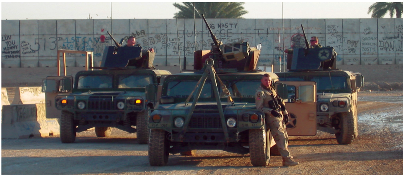
Three M1025 HMMWVs of the 518th Gun Truck Company with add-on armor kits waiting at CSC Scania.
