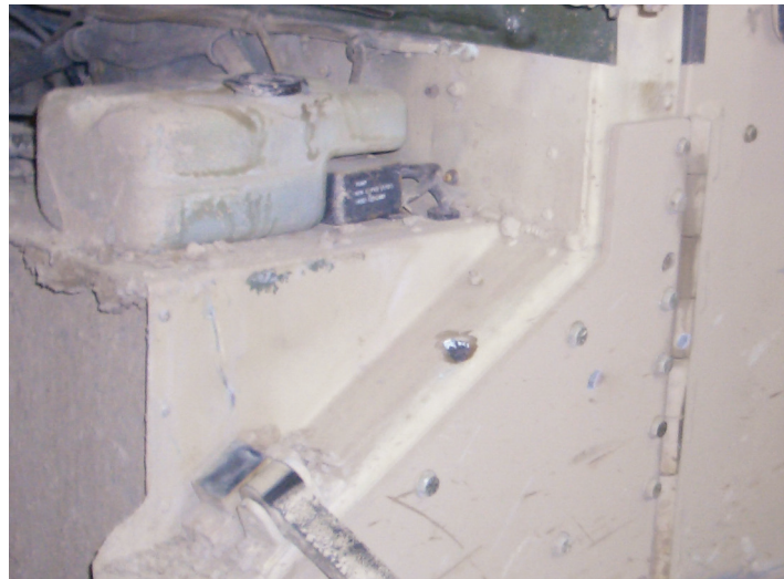
An AK round penetrated the gap between the add-on-armor and engine and struck Hubbard. Photo courtesy of Jonathan Kennedy
