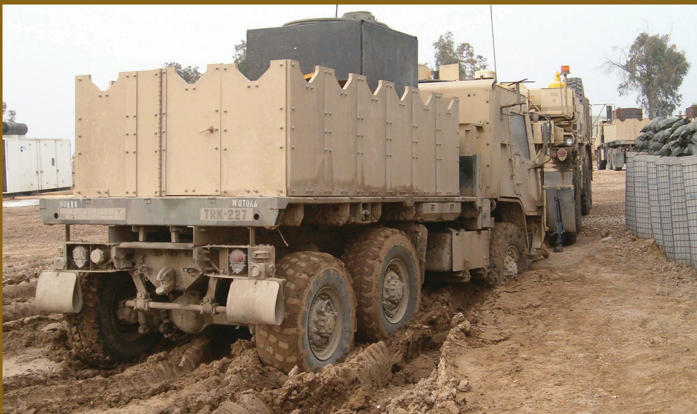
FMTV with Letterkenny gun box and Stewart and Stevenson cab armor kit. Photo courtesy of the 1544 Transportation Company
