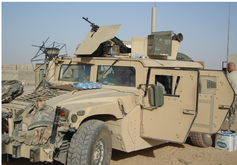
M1114 with SAW, Dukes electronic jammer and TACSAT. radio.
