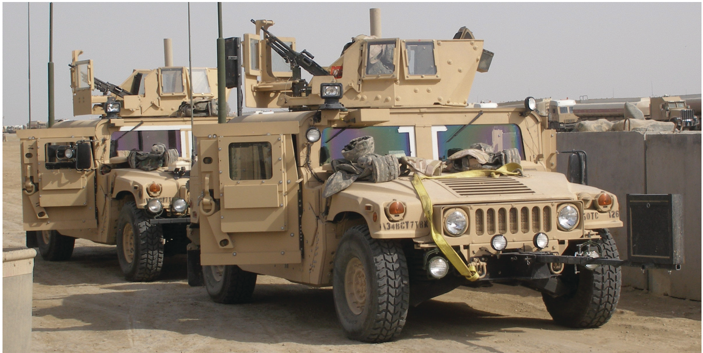
Lead M1114 with extra lights to illuminate the road ahead and the Rhino in the down position. Photo courtesy of Richard Killblane
