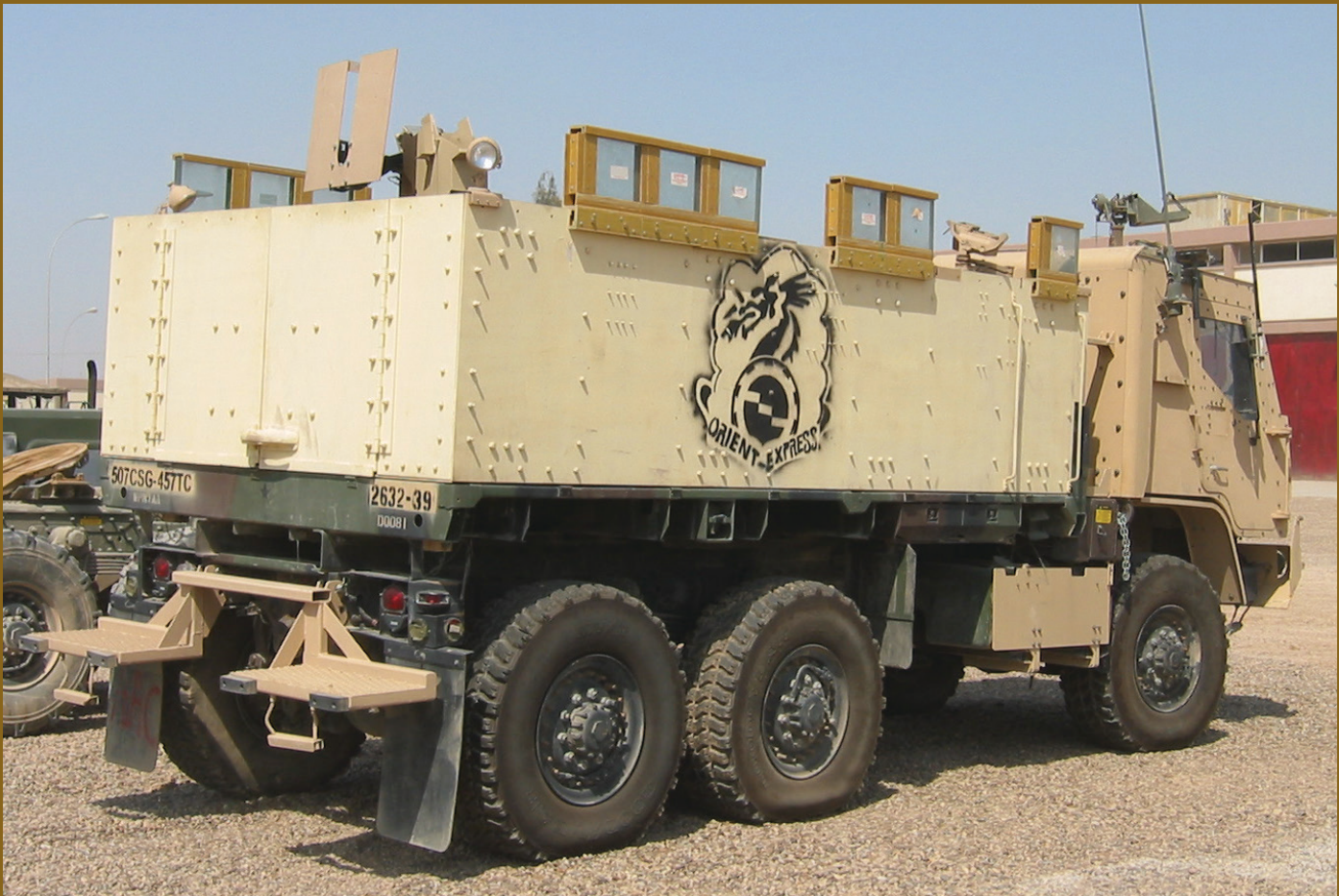
FMTV with Stewart and Stevenson gun box and cab armor kit. Photo courtesy of Richard Killblane
