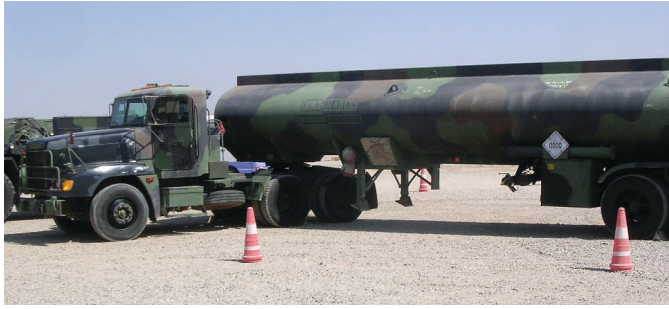
M915 tractor and 5,000-gallon tanker trailer of the 660th Transportation Company (POL), a sister company of the 724th POL also at Logistic Support Area Anaconda.
