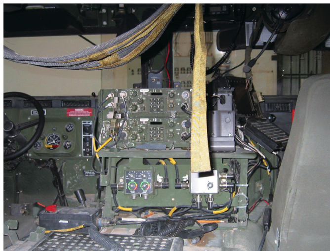
Interior of M1114 with double stacked SINCGARS and MTS. Photo courtesy of Richard Killblane
