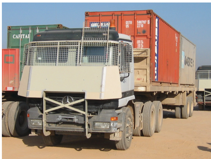
KBR Mercedes tractor with external armor.
