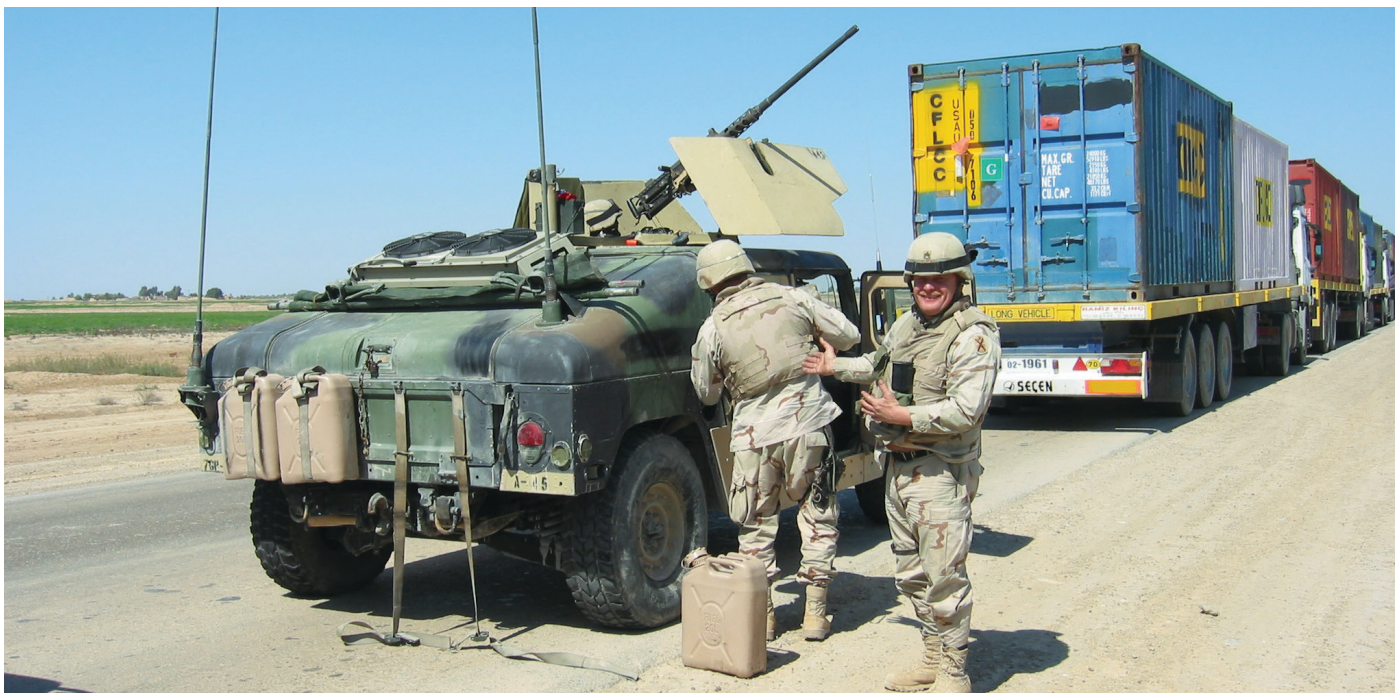
HMMWV of the 1-178th FA stopping to refuel on the eastern route because the up-armored HMMWVs consumed fuel faster and fuel tanks did not carry as much fuel as the M915s. Photo courtesy of Richard Killblane
