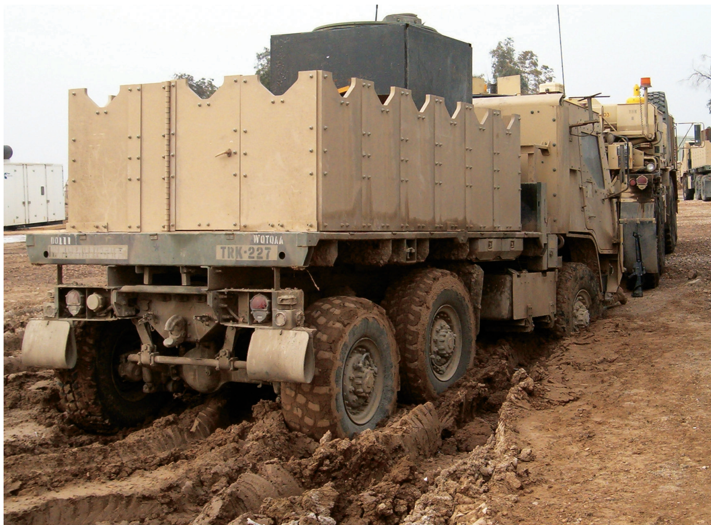
Letterkenny gun box on FMTV. Photo courtesy of 1544th Transportation Company
