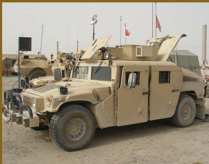
Top: M1114 with added ceramic plates and factory built bumper.
