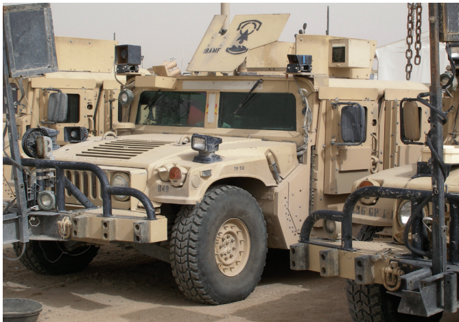
M1114 with Frag 5 door armor and Rhino 2 in the up position. Rhinos provided a heat signature ahead of the vehicle to detonate the IEDs triggered by motion detectors. The 1-121st FA had their 157th FA Brigade patch as the logo on their gun shields. Photo courtesy of Richard Killblane
