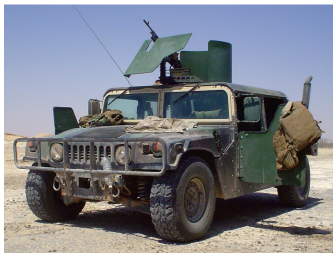
HMMWV gun truck of the 766th Transportation Battalion with first pattern add-on-armor kit, gun shield and turret armor. Photo courtesy of MAJ Ressel
