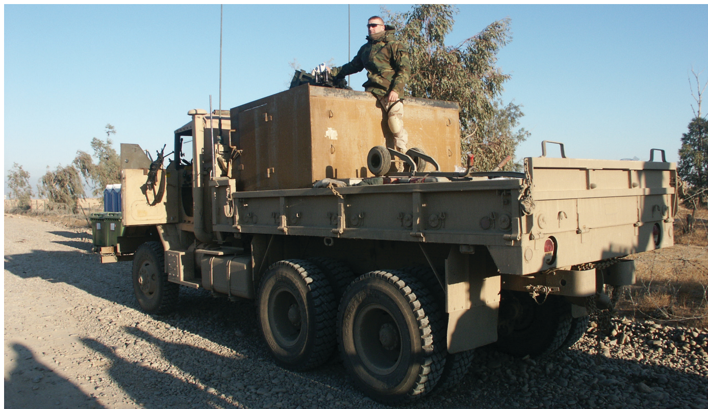
Rear view of "Big O" showing the fabricated steel gun box for the M2 .50 caliber machinegun. It also had mounts for M249 SAWs on the fabricated door armor. Photo courtesy of the 518th
