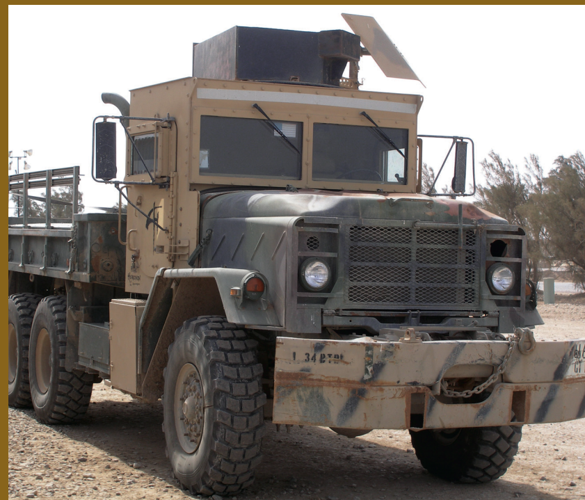
Top: Cab armor kit FMTV. Two Left: Cab armor kits for M915s. Right Bottom: Cab armor kit for M923 aka "Frankenstein Box"
