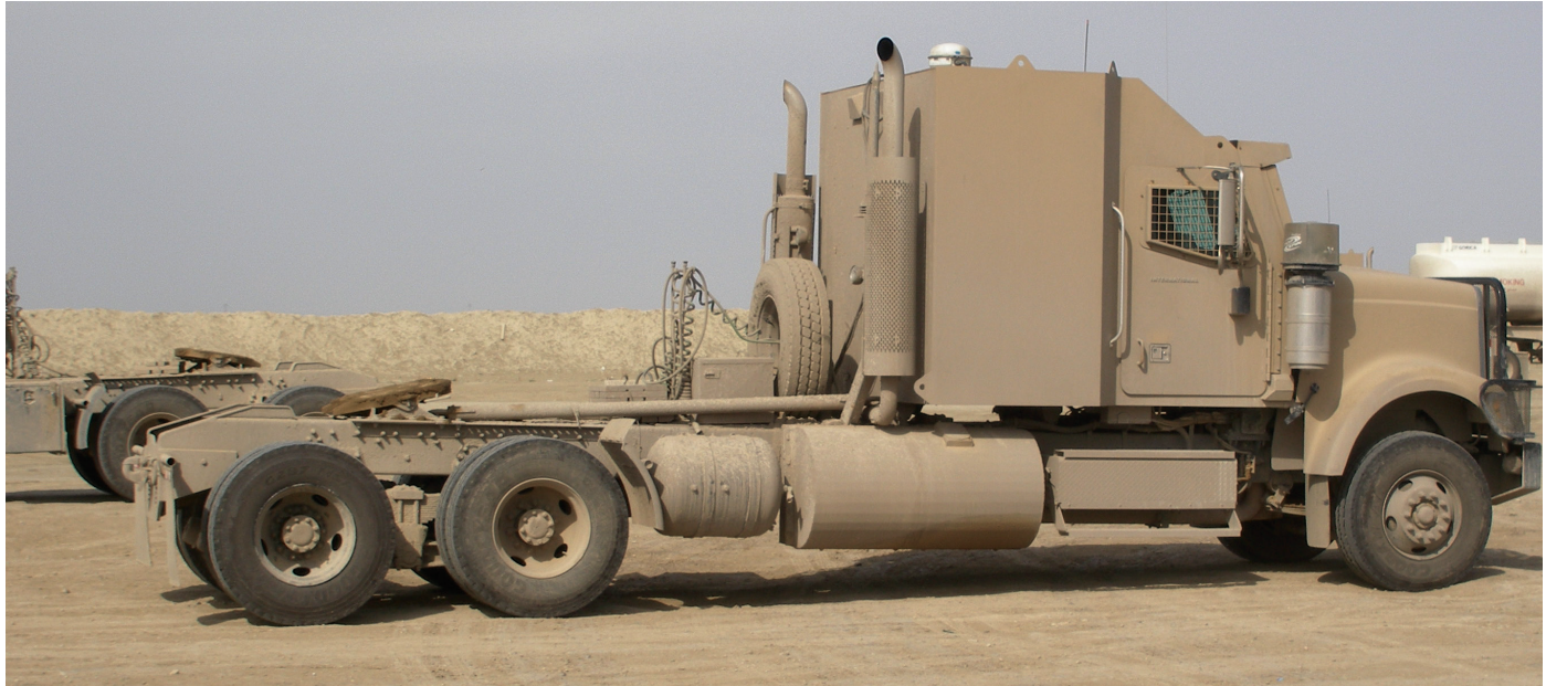
New armored cab of KBR tractors. Photo courtesy of Richard Killblane
