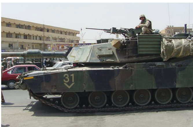
If the .50 caliber machine gun atop the turret could not defeat the threat then the 120mm main gun could.
