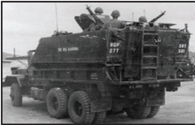
Figure 14. The Big Kahuna . APC hull mounted in a 5-ton truck.
